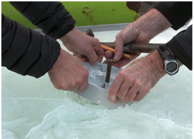
Figure 2. Oil pool depth and diameter were defined by a rubber baking form frozen into the ice at the surface. The form was easily removed from the ice at the beginning of the experiment.
