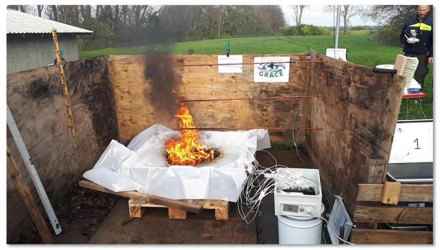
Figure 1 Overview of the burn experiment with ice pan and burning oil pool in the center.
