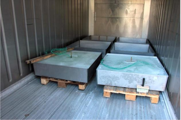
Figure 1. Simultaneous ice growth for multiple experiments in the cold room. Wires of the thermocouples measuring ice temperatures (green) can be seen to emerge at the left hand side of the tanks.
